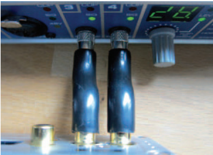
A short jumper between D/A and A/D transducers simulating operation without an interconnect cable.
