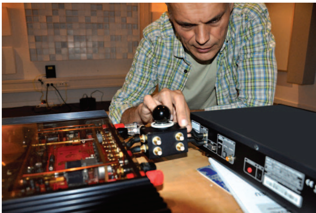
The Cable Comparator from specialists Wireworld allows small signal cable AB listening tests in comparison to a direct connection. Its electrical construction is absolutely uncompromising.
