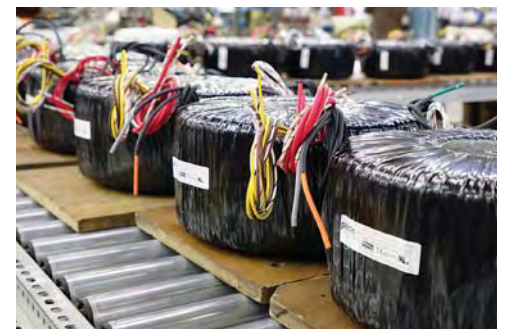
Torus Power's line-conditioning products are built around large and heavy toroidal transformers that filter out interference on the AC line, and supply large amounts of current to connected components on demand. Torus' parent company, Toronto-based Plitron Manufacturing, supplies power transformers to companies like Bryston and McIntosh, and also makes power products for hospitals, broadcasters and other industrial users.
